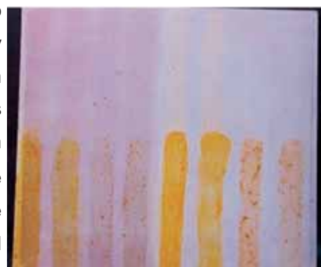
Spot tests on \text{TiO}_2 -coated ceramic tile. The top portion was exposed to fluorescent light.
