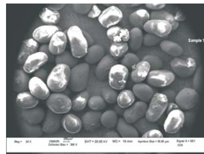
Near spherical NaCl crystals through new process that does not involve use of any additive
