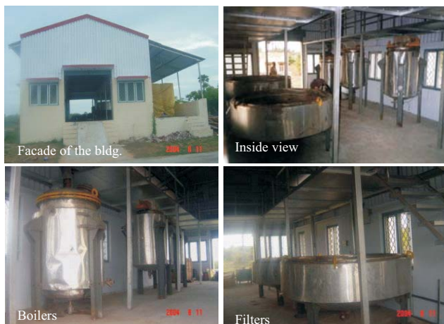
Pilot Plant shed constructed at Mandapam for processing of Agar and Carrageenan.
