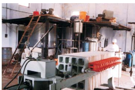
View of bench scale unit for recovery of SOP and MgO from bittern at Experimental Salt Farm of CSMCRI
