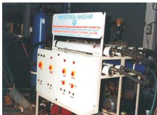
2-Stage 3000-4000 L (7-8 h operation) Seawater Desalination Plant at Nelmadur, Ramanathpuram for Treatment of groundwater having seawater salinity.
