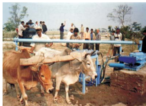
Oxen powered RO unit in Hasnabad, W. B
