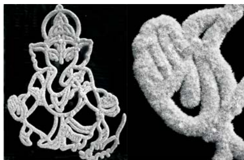
The picture depicts the innovation of encrustation of gypsum crystallites on a template. This innovation has its origin in the solar salt production process.
