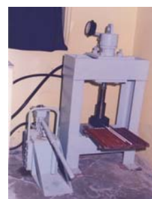
Hydraulic machine for extrude chalk
