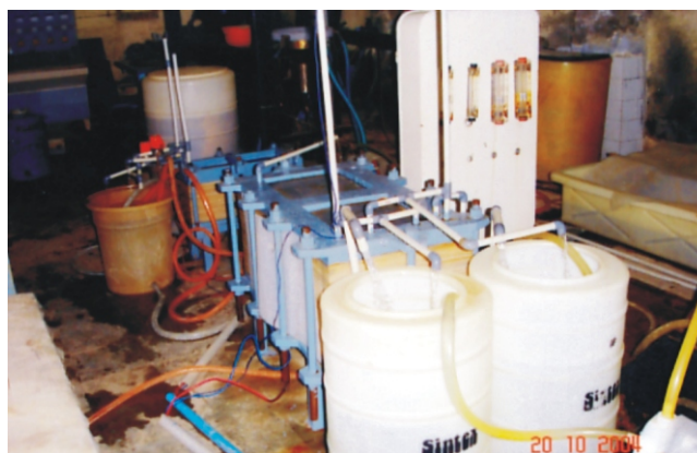
Sea water ED desalination plant being tested at CSMCRI, Bhavnagar
