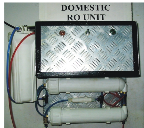
High pressure domestic RO desalination unit
