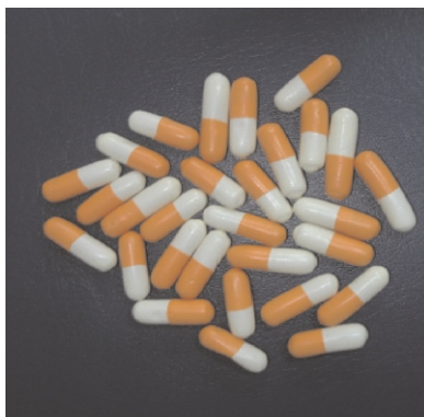
Semi-refined \kappa -carrageenan based hard capsule shells
