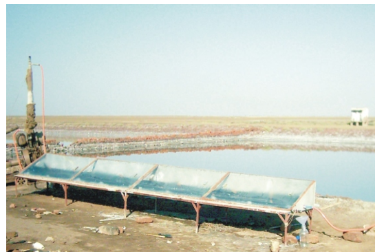
Waste heat augmented solar still in the CSMCRI salt farm
