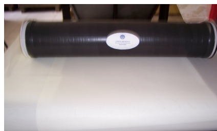
8040 spiral module rolled at CSMCRI
