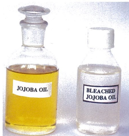
Jojoba oil as expelled (left) and after bleaching (right)
