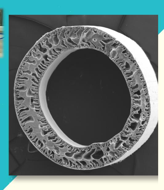
Polymer-inorganic hybrid; Outer Diameter = 1200-2450 μm Inner Diameter = 600 - 1700 μm;
